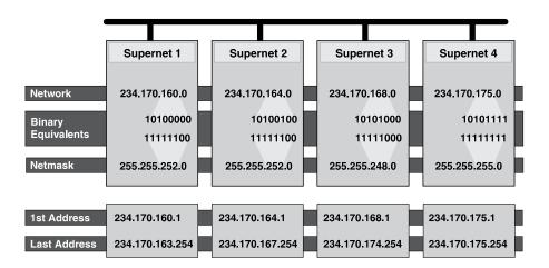
Supernets 1 and 2 each require four Class C networks, so they require a netmask with 2 zero bits  $(4 = 2^2)$  in the third octet. This yields a netmask of 255.255.252.0.
